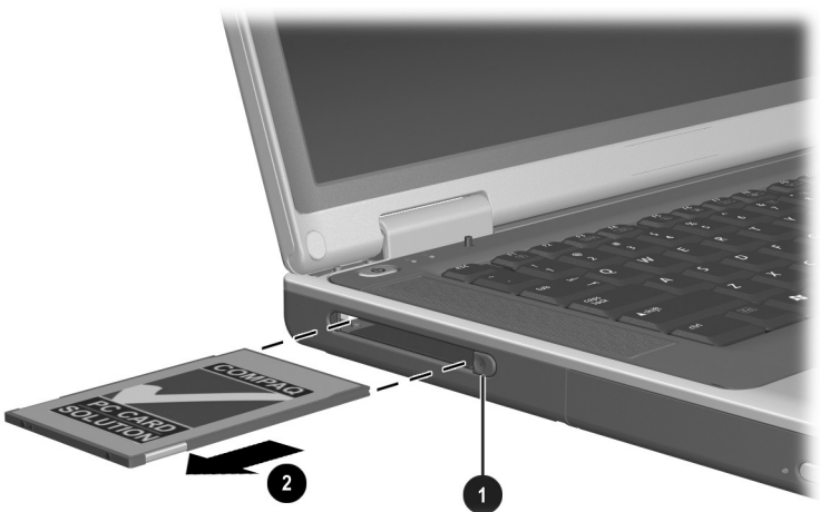
Removing a PC Card
